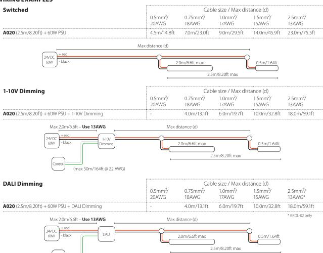
Note: This guide is produced from testing with KKDC approved power supplies or control gear.
